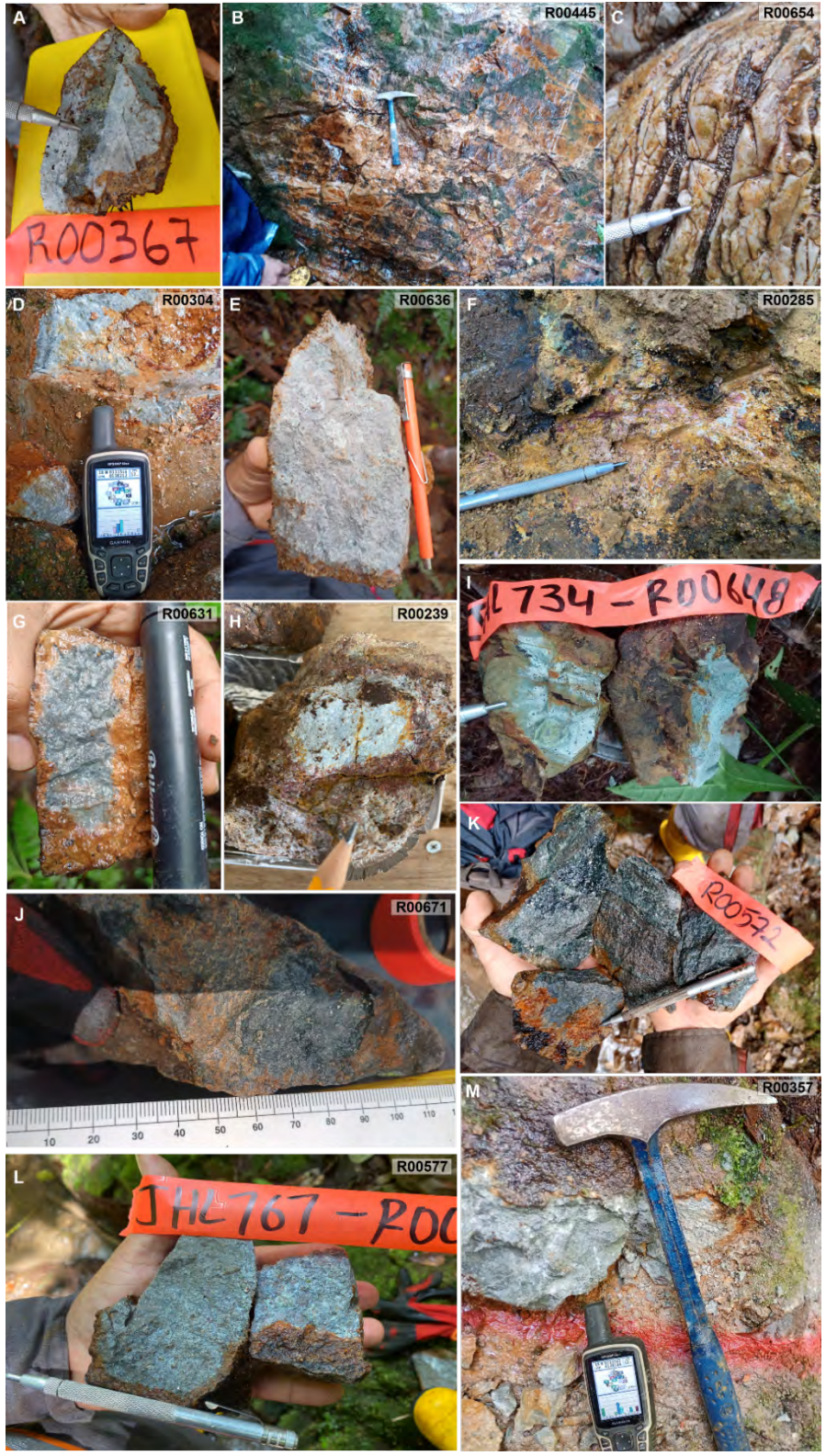
Figure 3. Highlighting rock samples in figure 2, showing the lithology, alteration and veining observed. A). Rock sample R00367 showing strong-sericite alteration in the upper part of the Mocoa porphyry with some remaining C-type veins (chalcopyrite dominant). B). Rock sample
